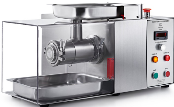
Caleva laboratory Variable Density Screw Extruder (Axial configuration)
