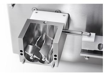
The torque generated is directly related to the consistency of the wet powder mass in the bowl. The instrument is programmed via the PC to mix the wet powder mass for user defined time periods. The instrument can also be programmed to prompt for binder additions at user-defined intervals. The use of a automatic binder addition module removes the requirement for user intervention during such a test. This will free up operator time for other activities during the process.
