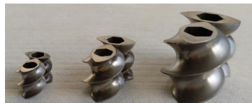
Figure 1. The three scales in this study: 11 mm, 16 mm and 24 mm sized twin-screws.
