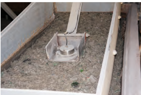
In sliding shoe for cullet (recycling glass)
