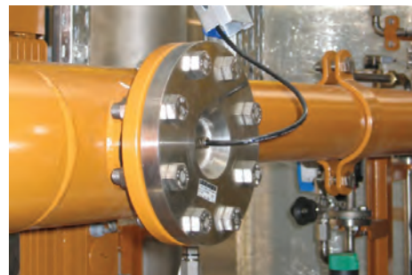
With DN 80 flange for diesel, oil and other emulsions
