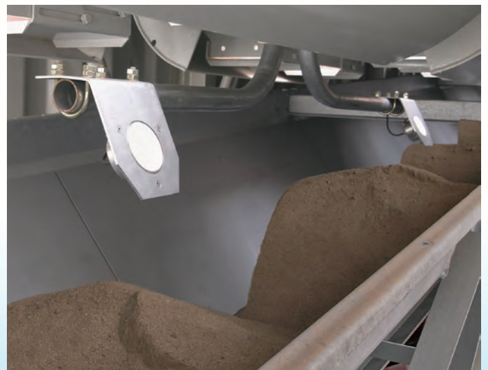
Moisture measurement of sand in a concrete mixing plant
