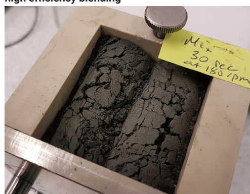
Mixing at high speed for about 30 seconds offers a high efficiency blending
