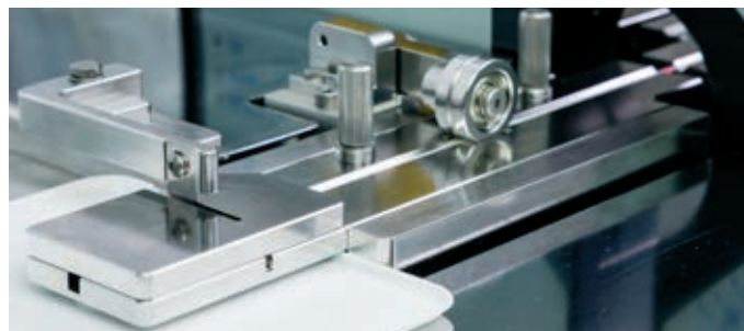
Laser based take-off and cutting system
