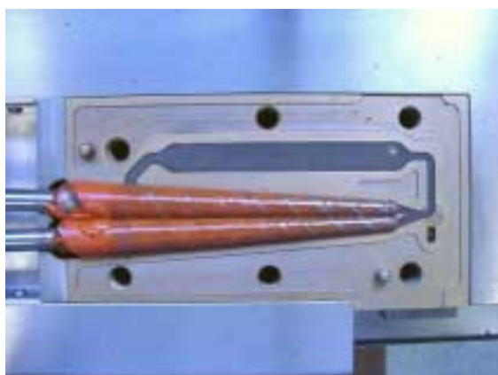
Figure 2: Co-rotating screws: a): PE melt, b) Asaclean (PS cleaning compound) + Remafin orange duration of the test t = 90 s, test conditions like in Figure 4.
