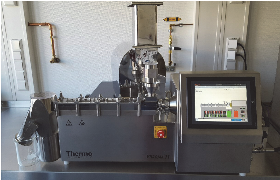
Fig. 2: Process set-up for dry granulation: Pharma 11 Twin-Screw Extruder with granulation kit.
