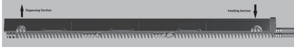
Fig. 1: Set up of screws and barrel used for the scale up experiments on the Pharma 11, Pharma 16 and Process 24. At the feeding section the Soluplus® is added as well as the pigment is added at a given time T_0 . The degassing section at the left hand side is an atmospheric degassing to allow water vapor to evaporate out of the polymer.
