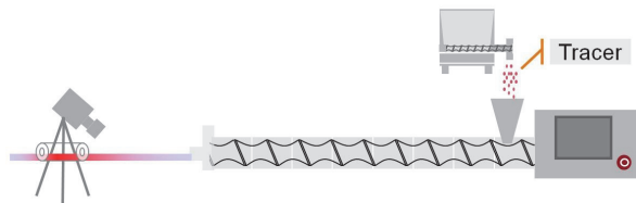
Fig. 2: Residence time distribution measurement set up
