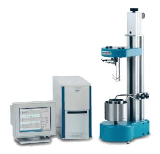
The viskomat NT is a versatile rotational viscosimeter for determing the workabilty of finegrained building materials such as cement paste, mortar, fine concrete, plaster etc. with a maximum particle size of 2 mm. You can obtain information on:
