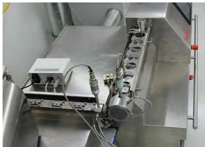
Figure 1: Set-up of twin-screw extruders for co-extrusion.
