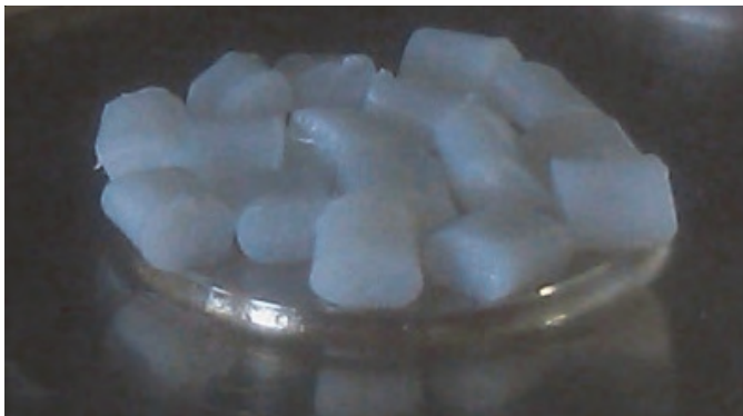
Fig. 3: Extrudate pieces placed on the lower plate of the measuring geometry for melting and subsequent loading and trimming.
