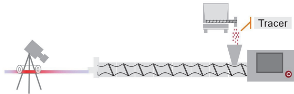
Fig. 2: Residence time distribution measurement set up
