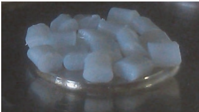
Fig. 3: Extrudate pieces placed on the lower plate of the measuring geometry for melting and subsequent loading and trimming.
