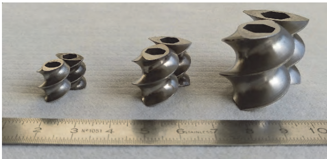
Fig. 3: The three scales in this study: 11 mm, 16 mm and 24 mm sized twin-screws.
