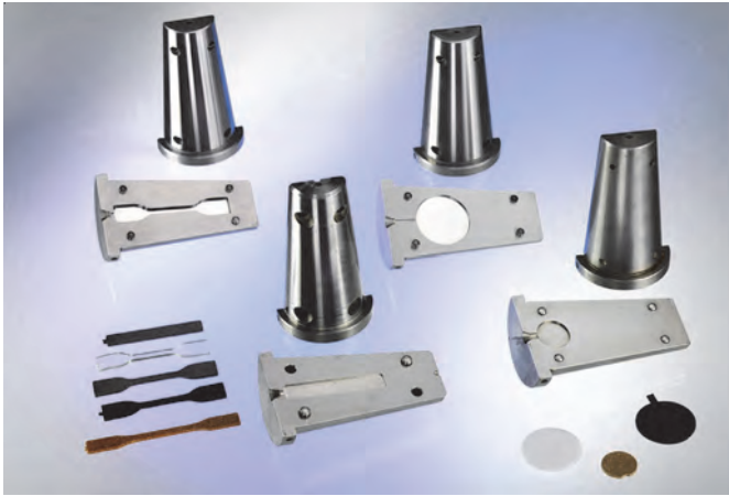
Fig. 5: HAAKE MiniJet molds with injection molded samples of different shape and size.
