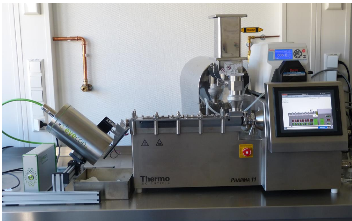
Figure 8 - Eyecon 2 Particle Analyser with Integration Device in-place on Pharma 11 Extruder in Granulation Mode (View 3)
