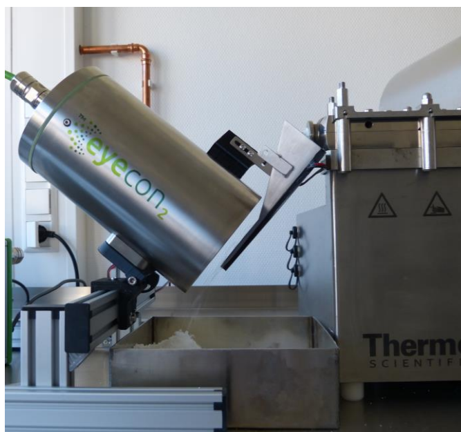
Figure 7 - Eyecon 2 Particle Analyser with Integration Device in-place on Pharma 11 Extruder in Granulation Mode (View 2)
